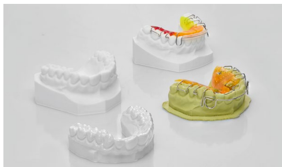
Fig. 4 Finished orthodontic models directly after printing
